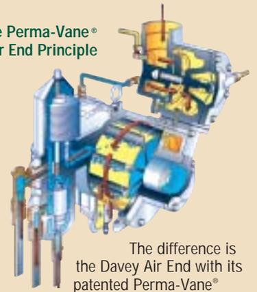
The difference is the Davey Air End with its patented Perma-Vane®
